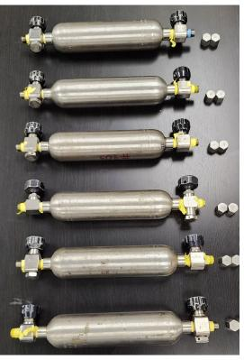
Figure 3. NGL samples are provided in sampling cylinders. A few grams of sample is mixed with an equal mass 10-mM HCl (aq) for extraction.
