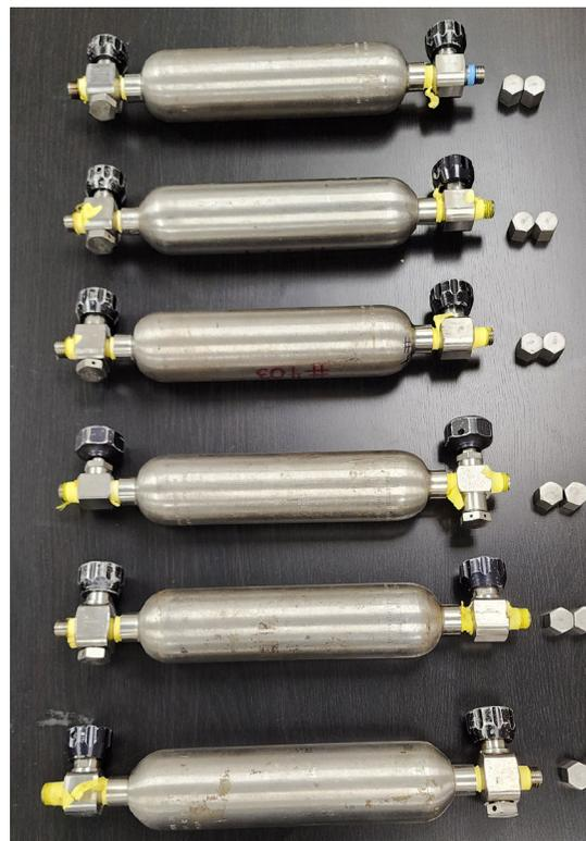
Figure 3. NGL samples are provided in sampling cylinders. A few grams of sample is mixed with an equal mass 10-mM HCl (aq) for extraction.
