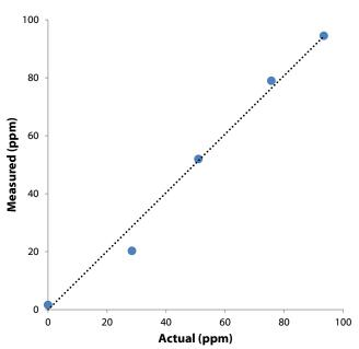
The results are shown in Figure 4. The concentration of extracted dithiazine from serial dilutions of a 129-ppm sample followed the expected curve.
