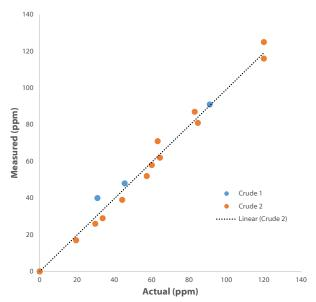
Figure 3. MEA-triazine content in two different crude oil samples. The samples were spiked with MEA-triazine to a known concentration, and then diluted to various levels. The triazine was extracted and measured.
